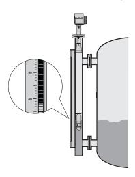
The BM 26 W has a float and indicating tube for indicating level on a highly visible column of yellow and black rotating flaps. No power is needed. It is also possible to fit limit switches, if you choose this option. Ex approval is optional.
